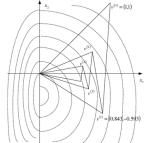
Nelder-Mead operates a series of contractions and converges to a nonstationary point on McKinnon functions which are convex and continuously differentiable (plot from [12]).
