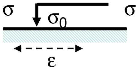
$$\dot{\varepsilon} = \begin{cases} 0 & \text{si } |\sigma| < \sigma_0 \\ 0, & \text{si } |\sigma| = \sigma_0 \text{ et } \frac{d}{dt}|\sigma| < 0 \\ \lambda \frac{\sigma}{|\sigma|}, \lambda \in \mathbb{R}^{*+} & \text{si } |\sigma| = \sigma_0, \frac{d}{dt}|\sigma| = 0 \end{cases}$$
