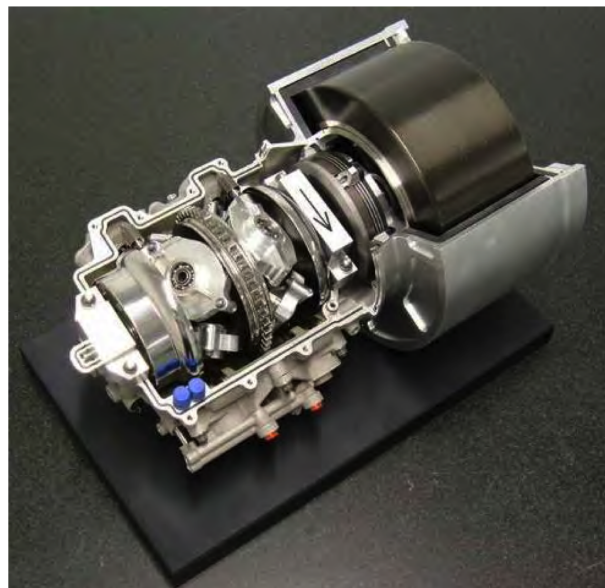
FIGURE 6 – Volvo KERS system Flywheel hybrid systems http://www.racecar-engineering.com/articles/f1/flywheel-hybrid-systems-kers/
