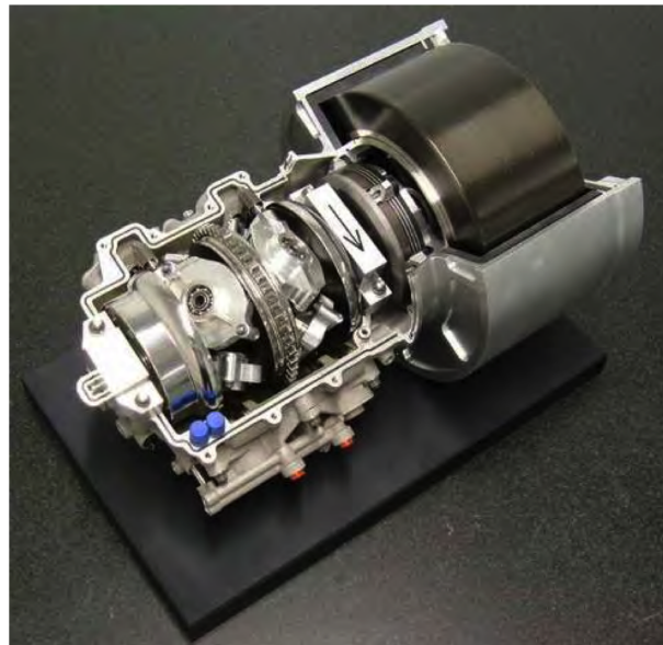
FIGURE 6 – Volvo KERS system Flywheel hybrid systems http://www.racecar-engineering.com/articles/f1/flywheel-hybrid-systems-kers/ (dernier accès : 12/11/2021)
