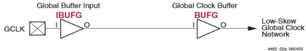
a. Global Buffer Inputs and Clock Buffers Drive a Low-Skew Global Network in the FPGA
