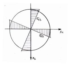
Figure 4.7: Stress in a twisted circular section.
