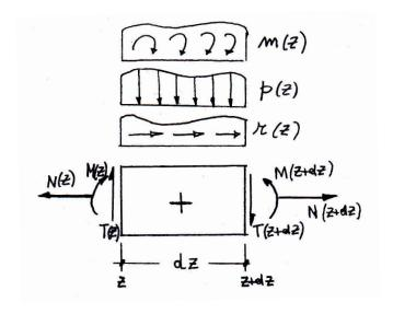
Figure 5.1: General sketch for the rod's balance equations.
