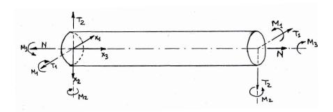
Figure 4.2: Conventions for the signs of the internal actions.
