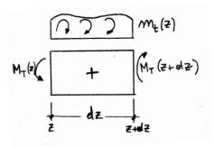
Figure 5.3: Scheme for the torsion of a rod.
