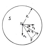
Figure 4.6: Torsion of a circular section.
