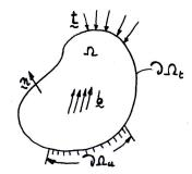
Figure 2.6: Scheme of the boundary conditions.
