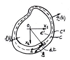
Figure 4.10: General scheme for the Bredt's solution.
