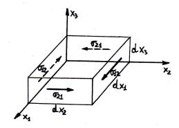
Figure 2.5: Reciprocity of the shear stresses.
