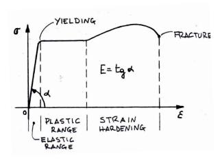
Figure 3.1: Typical  $\sigma - \varepsilon$  diagram.
