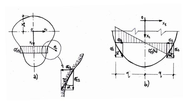
Figure 4.14: The shear stresses in the Jourawski solution.
