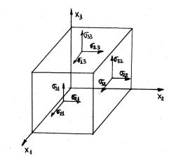
Figure 2.3: The components  $\sigma_{ij}$ .
