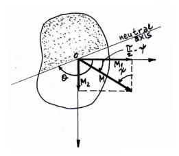
Figure 4.5: Biaxial bending.
