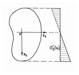
Figure 4.3: Variation of  $\sigma_{33}$  on a cross section.
