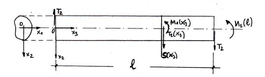
Figure 4.13: Scheme for the analysis of the shear.
