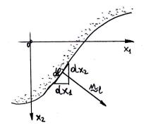
Figure 4.8: Outward normal  $\mathbf{n}_l$  in a generally shaped section.
