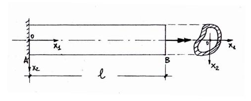
Figure 4.12: Scheme for the calculation of the twist angle with the Bredt's solution.
