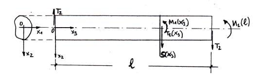
Figure 4.13: Scheme for the analysis of the shear.
