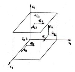
Figure 2.3: The components  $\sigma_{ij}$ .
