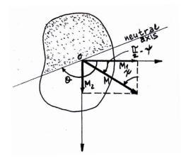
Figure 4.5: Biaxial bending.
