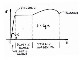
Figure 3.1: Typical  $\sigma - \varepsilon$  diagram.
