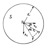
Figure 4.6: Torsion of a circular section.
