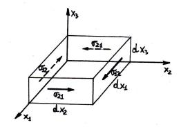
Figure 2.5: Reciprocity of the shear stresses.
