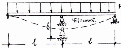
17. Make the same, loading now the rod uniquely by a thermal load of the type  $t^- = -t$ ,  $t^+ = +t$ .
