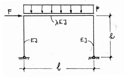
19. Calculate the total displacement of point  $C$  for the structure in the figure using the dummy load method.
