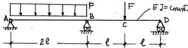
13. Solve the previous problem with the span  $AB$  now loaded by a through the thickness linear variation of the temperature of the type  $t^- = -t$ ,  $t^+ = +t$ .
