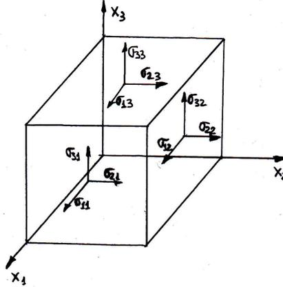
Figure 2.3: The components  $\sigma_{ij}$ .
