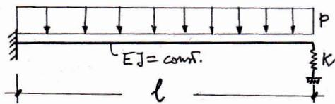
15. Make the same, loading now the rod uniquely by a thermal load of the type  $t^- = -t$ ,  $t^+ = +t$ .
