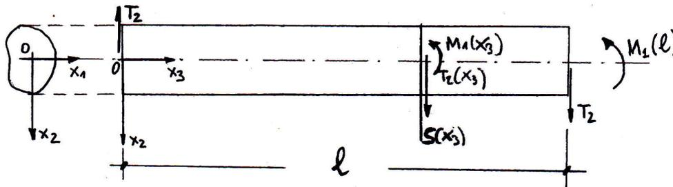
Figure 4.13: Scheme for the analysis of the shear.
