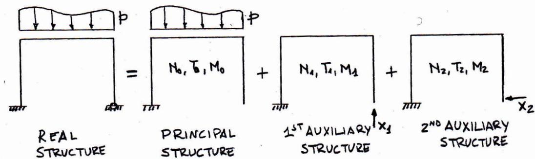
Figure 5.4: Scheme for the analysis of hyperstatic rod structures.
