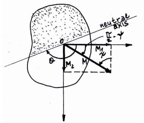
Figure 4.5: Biaxial bending.
