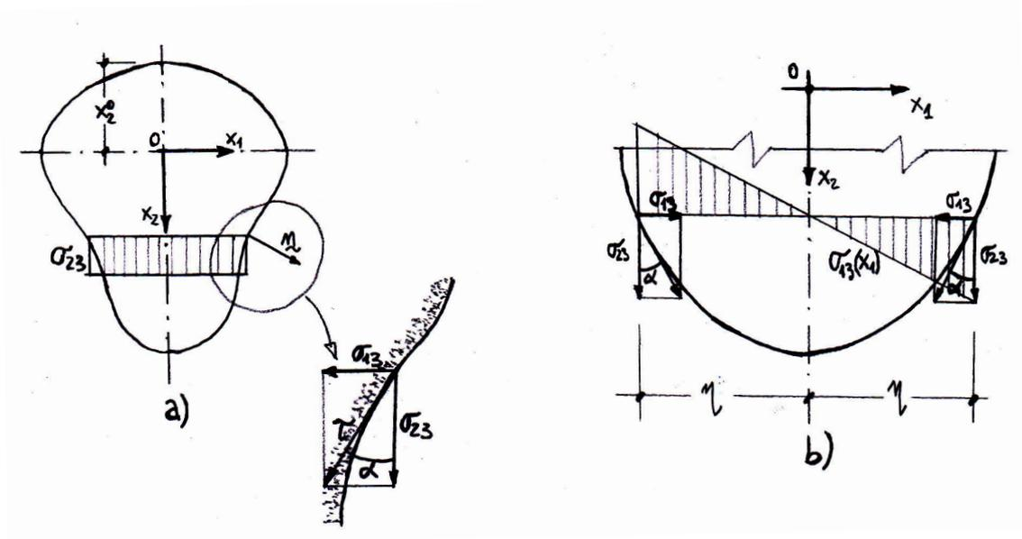
Figure 4.14: The shear stresses in the Jourawski solution.
