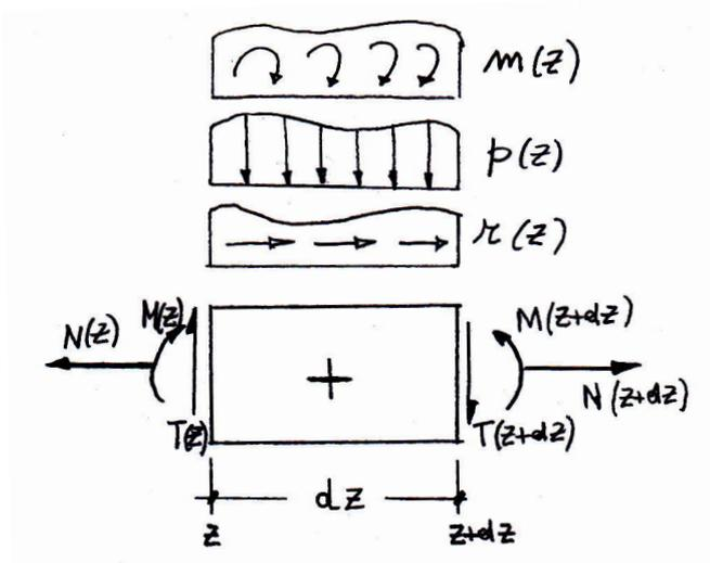
Figure 5.1: General sketch for the rod's balance equations.
