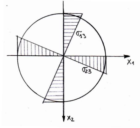
Figure 4.7: Stress in a twisted circular section.
