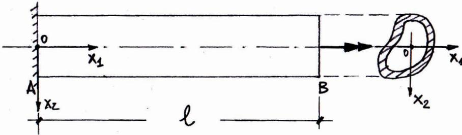
Figure 4.12: Scheme for the calculation of the twist angle with the Bredt's solution.
