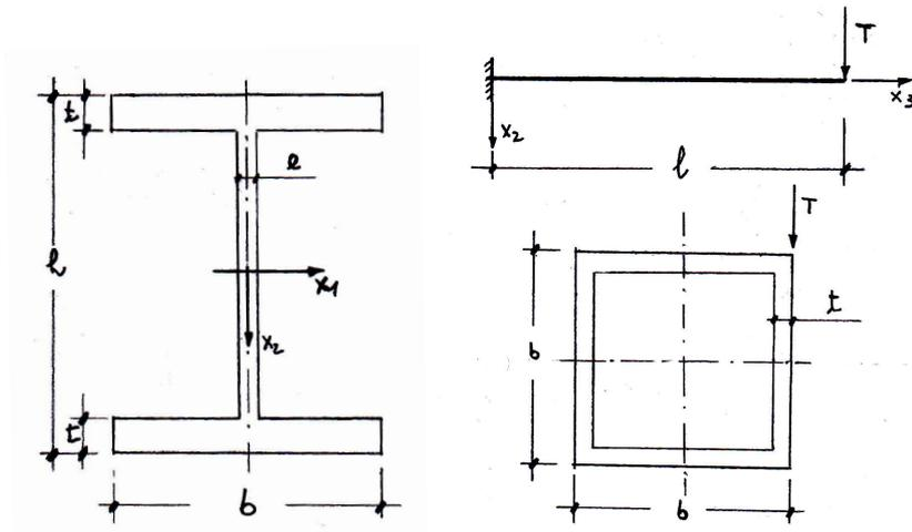
23. Calculate the stress state for the beam in the figure, having a hollow square section. Then, check the safety of the structure using the HHVM criterion, knowing that the limit stress is  $\sigma_0$ . Data:  $T = 4$  KN,  $b = 200$  mm,  $t = 6$  mm,  $l = 4$  m,  $\sigma_0 = 160$  MPa.
