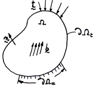
Figure 2.6: Scheme of the boundary conditions.
