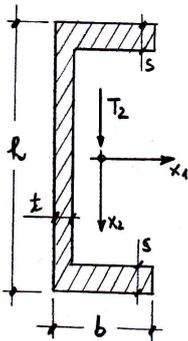
22. A section of steel with section I as in the figure is submitted to a shear force  $T_2$  and a bending moment  $M_1$ . Knowing the yielding stress  $\sigma_0$ , determine if the section can withstand the applied actions using the HHVM criterion. Data:  $h = 400$  mm,  $t = 12$  mm,  $e = 8$  mm,  $b = 200$  mm,  $T_2 = 2000$  KN,  $M_1 = 50$  KNm,  $\sigma_0 = 160$  MPa.
