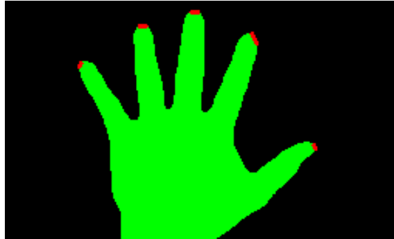
Extremities (slightly dilated) of the hand image. The result is the same if the geodesic center or the centroid is used.
