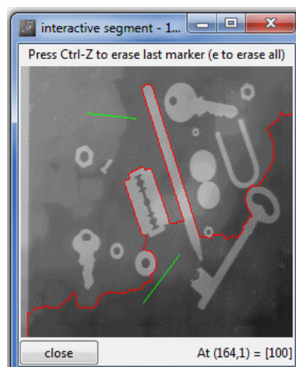
Only two markers have been used. Both are in the background. Therefore, the image is divided into two catchment basins and the watershed line is not very helpful.
