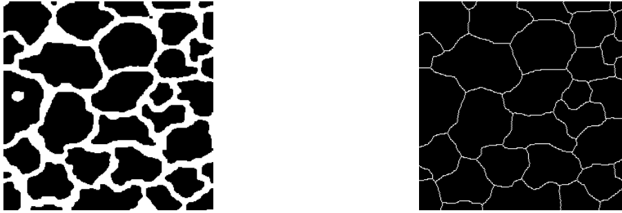
Watershed (right image) of the indicator function of the initial complemented set (left image).
