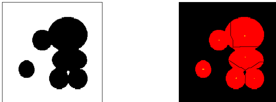
Initial disk image (left) and geodesic influence zones (in red) of the components of the ultimate erosion (yellow).
