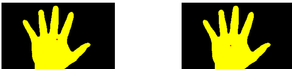
Geodesic center of the hand image (left), centroid (right). Due to the palm of the hand, the position of the two centers is quite different.
