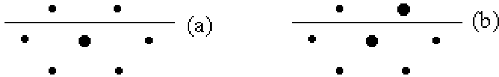
(a) initial picture, (b) linear dilation at 60^\circ , the point exits the field and is lost.
