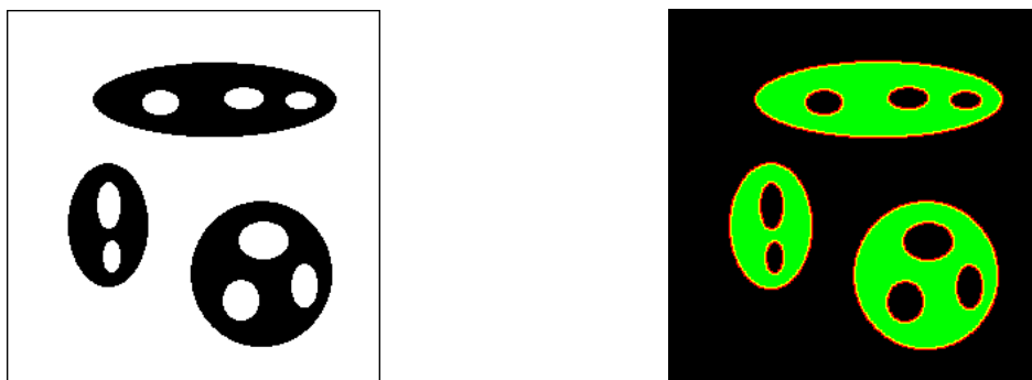
The two_three_holes image (left) and the internal (yellow) and external (red) contours.
