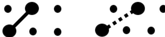
On the square grid (left), the two points are neighbors (one component). On the hexagonal grid (right), the same configuration is cut into two components (non neighbor points).
