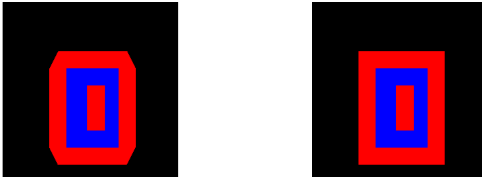
Dilation of size 25 of the shape image with an hexagon (left), dilation of size 25 with a square (right).
