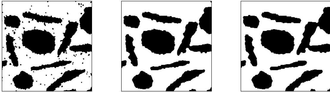
Black (start with a closing) alternate filters of noise image with hexagons of size 1 (left), 3 (middle) and 4 (right).
