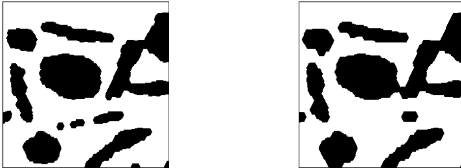
Alternate filters starting by a closing of size 1 with a step equal to 2 (left) or to 3 (right).
