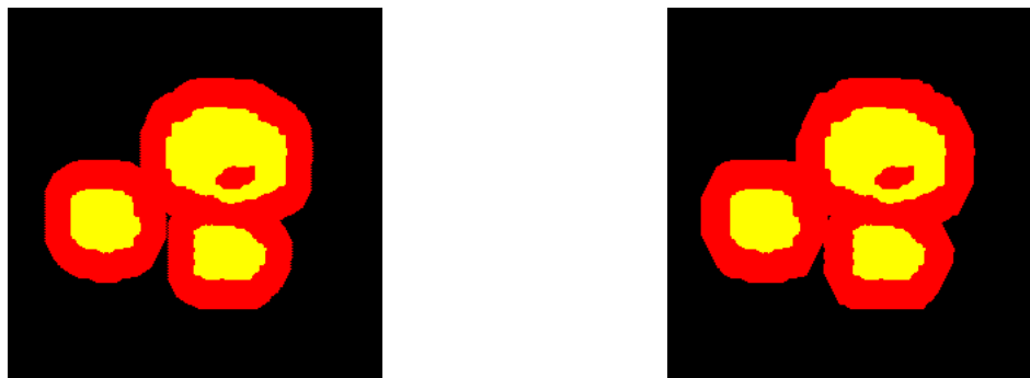
Dodecagonal dilation of size 20 of the objects image (left). This transformation can be compared to the hexagonal dilation of same size (right).
