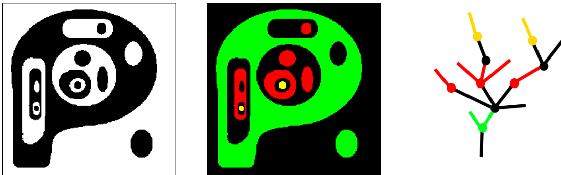
Left: homotopy image. Middle: homotopy tree represented by an image; the connected components of same color belong to the same level of homotopy. Right: corresponding homotopy tree; the black branches represent holes.
