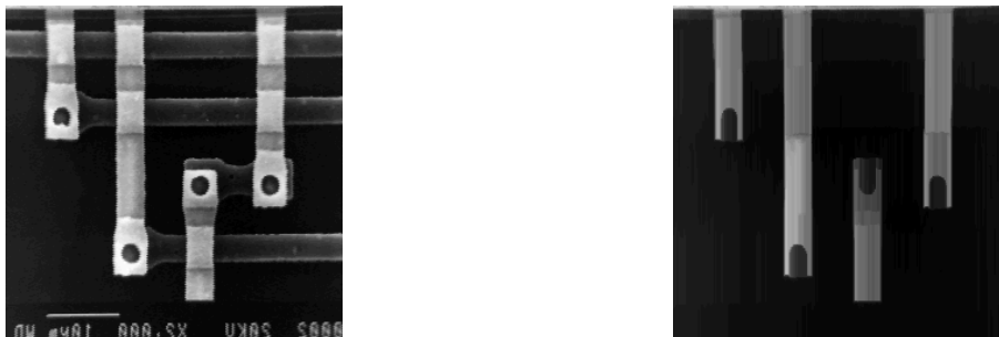
Opening by a vertical segment of size 50 (right) of the circuit image (left). The vertical features are more or less preserved, the horizontal ones are filtered.
