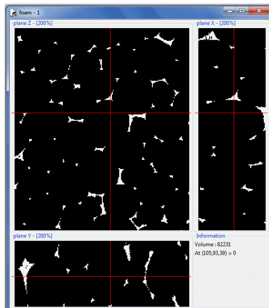
In PROJECTION mode, the three projections of the 3D image are displayed and it is possible to navigate inside it by moving the mouse cursor.
