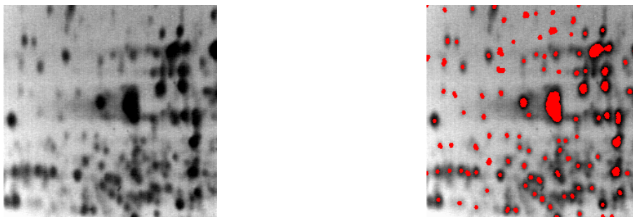
Minima (right) of the electrop image (left) filtered with an alternate sequential filter of size 2 starting with an hexagonal opening.
