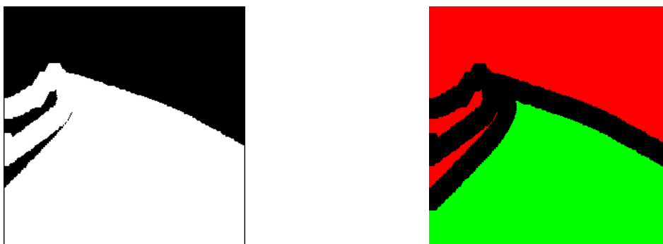
The non rebuilt marker in the previous step is added to the previous step (left). This set defines the outside marker in red whilst the green connected component is the marker of the road (right).
