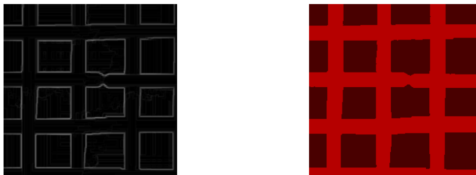
Gradient of the raster image (left) and result of the watershed transform (right).
