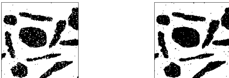
Left image, triangular opening followed by a triangular closing. Right image, the order of operations is reversed.
