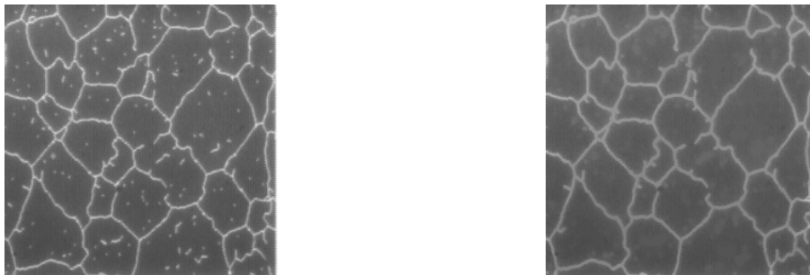
alumine image (left) and removal of the inclusions considered as white holes in the image (right).
