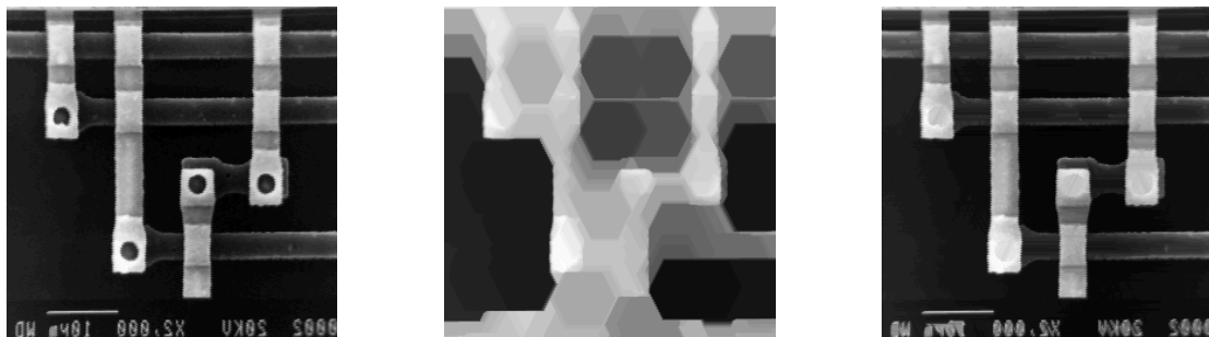
Initial image (left), hexagonal closing of size 20 (middle), sup of linear closings of size 20 (right).
