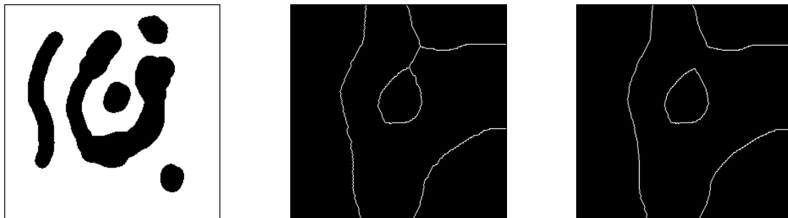
Initial image (left), SKIZ obtained by thickenings (middle), SKIZ obtained by watershed of the distance function (right). A false separation appears in the SKIZ by thickenings. This boundary is included inside the same influence zone.
