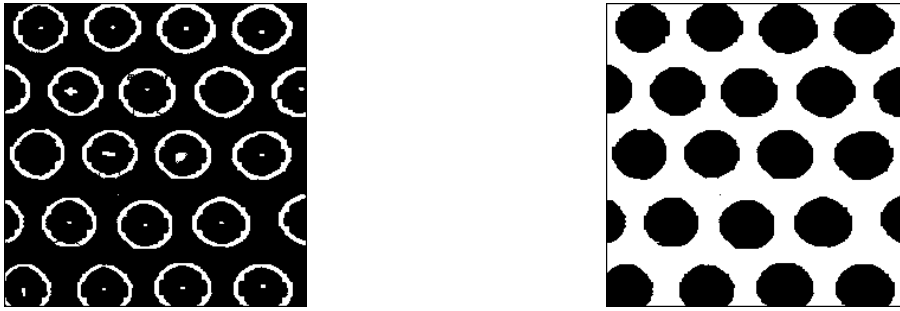
Filling the fibers of the boron2 image (left) with the closeFibers procedure (right).
