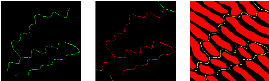
Left: end points (red) of the dislocations (green). Middle: the simple arcs touching the edge and connected to the end points are added. Right: boundaries of the cells containing stacked lamellae.
