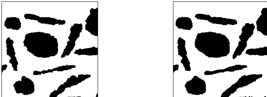
Full alternate sequential filter of size 4 of the noise image with a triangular structuring element, starting with an opening (left) and a closing (right).
