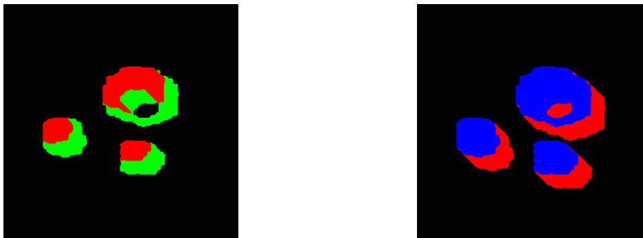
Linear erosion of the objects image (left) of size 15 in direction 4 of the square grid (the eroded set in in red). Linear dilation (right) of size 15 in direction 8 of the square grid (the initial set is in blue, the dilation adds the red points).
