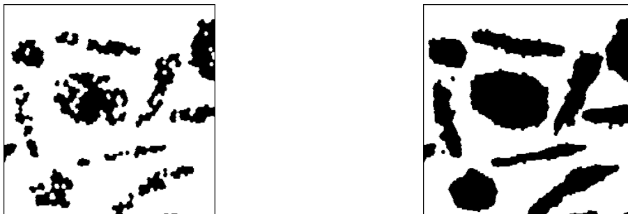
Full alternate filter of size 2: left image, the filter starts with an hexagonal opening, right image, the filter starts with an hexagonal closing.
