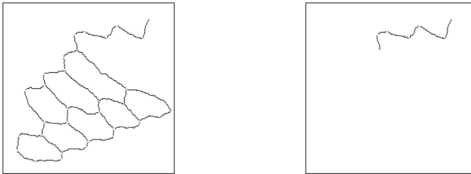
Arcs touching the edge are removed (left), arcs not surrounding or inside inner influence zones are extracted, they belong to dislocation lines (right).
