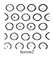
The *boron1* and *boron2* images represent boron fibers in a composite material. These fibers reinforce the mechanical resistance of the material. The resistance increases in proportion of the regularity of the fibers layout. Therefore, during industrial production, they are as far as possible placed according to a regular hexagonal network. However, irregularities occur.
