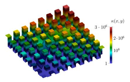
Figure 8.6: Diffusivity  $\kappa$  used for the two-dimensional weak scaling experiments with channels and inclusions.
