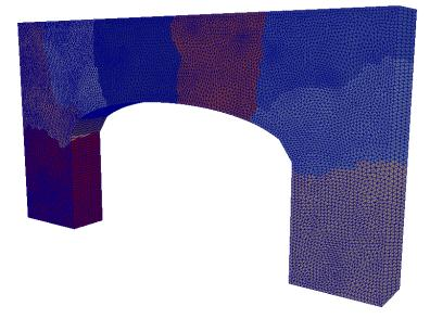
Listing 8.2: ./PARALLEL/FreefemProgram/elasticity-3d.edp This geometry is partitioned and distributed among the MPI processes.
