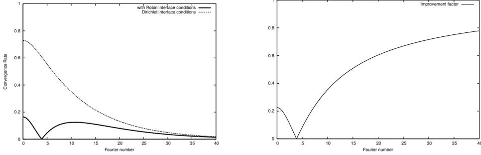
Figure 2.2: Left: Convergence factor (dotted line: Dirichlet ICs, solid line: Robin ICs) vs. Fourier number. Right: Improvement factor due to Robin interface conditions (2.8) vs. Fourier number
