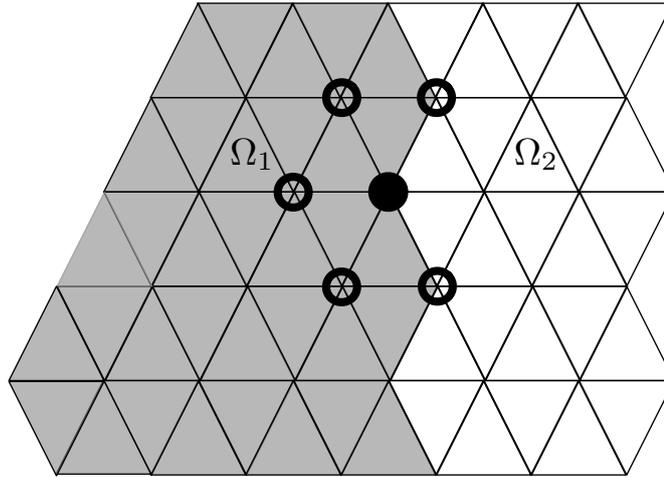
Figure 2.5: Stencil for the outward normal derivative  $(\partial u_1/\partial \mathbf{n}_1)$  at the interface between two non overlapping subdomains  $\Omega_1$  and  $\Omega_2$
