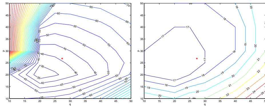
Figure 2.10: Number of iterations needed to achieve a certain precision as function of the optimization parameters  $p$  and  $q$  in the zeroth order transmission conditions, for the iterative algorithm (left) and for the Krylov accelerated algorithm (right). The star denotes the optimized parameters  $p^*$  and  $q^*$  found by our Fourier analysis
