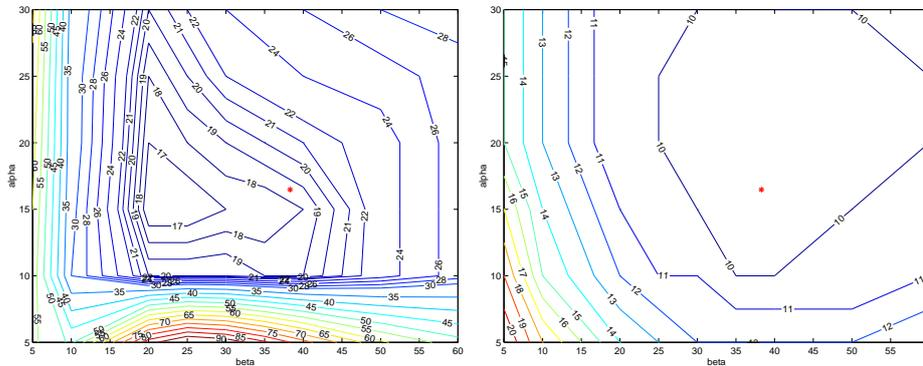
Figure 2.11: Number of iterations needed to achieve a certain precision as function of the optimization parameters  $\alpha$  and  $\beta$  in the second order transmission conditions, for the iterative algorithm (left) and for the Krylov accelerated algorithm (right). The star denotes the optimized parameters  $\alpha^*$  and  $\beta^*$  found by our Fourier analysis
