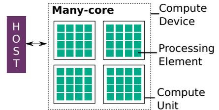
Figure 4: OpenCL platform model on many-core SoC.
