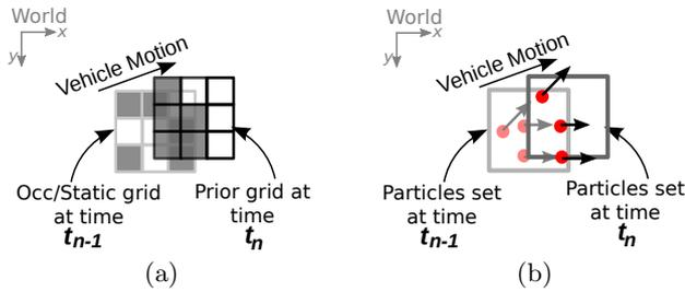
Figure 3: (a) Prior grids propagation. (b) Particles propagation.
