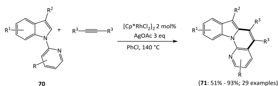
Scheme 37. Synthesis of 71 between N -pyridylindoles 70 from a dehydrogenative coupling reaction.
